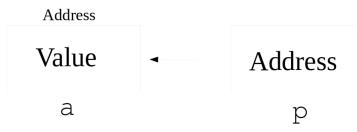
Figure 3 The pointer p points to the variable a.
